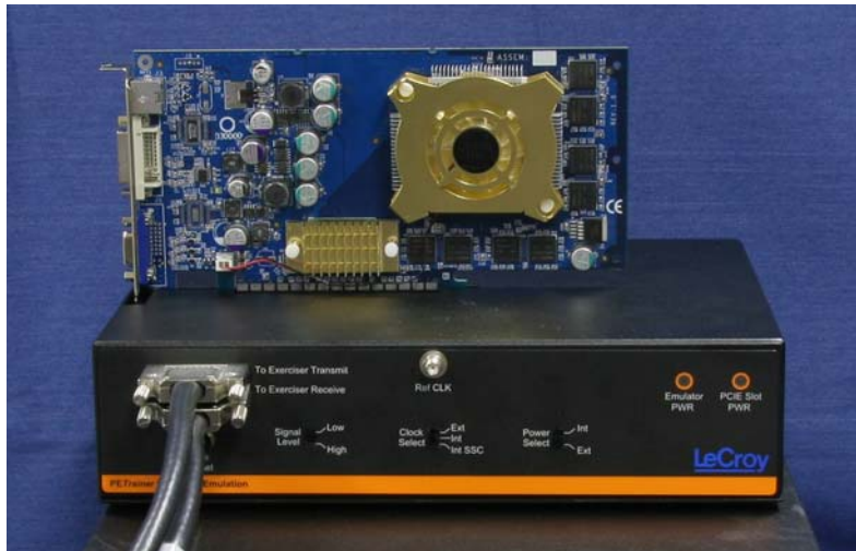
Figure 3.11 Host Emulation Test Fixture with a PCI-E Graphics Card on Top
