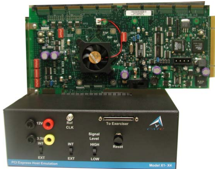
Figure 3.6 Host Emulation Test Fixture with DUT Card on Top
