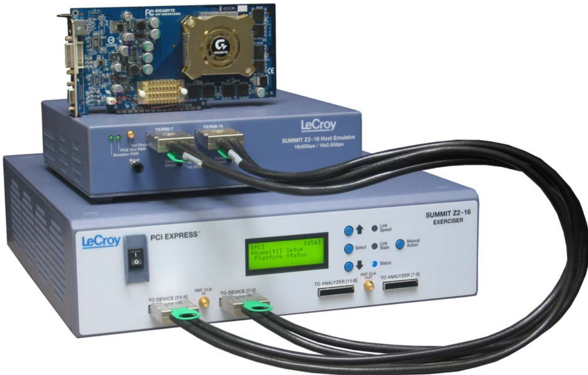
Figure 3.14 PETrainer Summit Z2-16 Exerciser (bottom) connected to a Host Emulator adapter (top). The Host Emulator has a PCI Express graphics card inserted.
