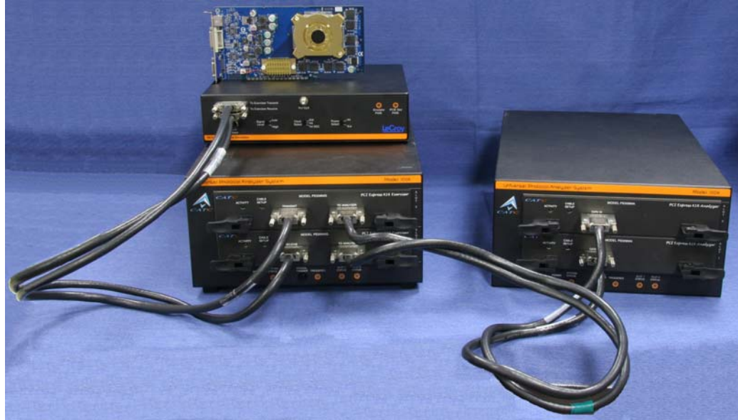
Figure 3.10 PETrainer EML (bottom left) connected to a Host Emulator adapter (top) and a PETracer EML Analyzer (right). The Host Emulator has a PCI Express graphics card inserted.
