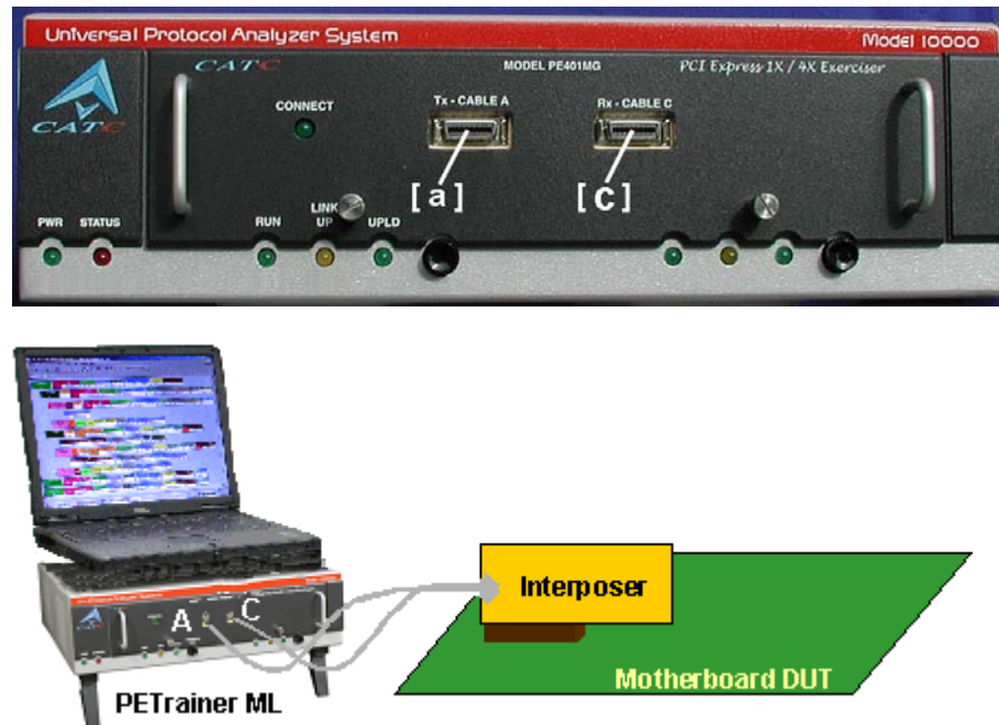
Figure 3.7 PETrainer ML Front Panel showing where Connectors A and C Attach
